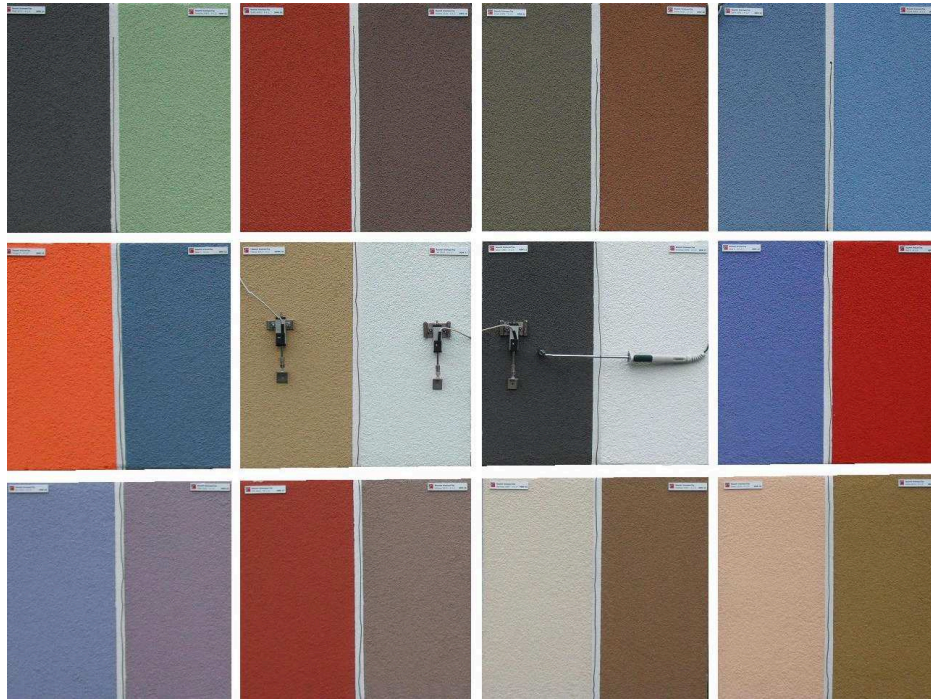
Fig. 1. Arrangement of tested samples ETICS into the testing patterns.
