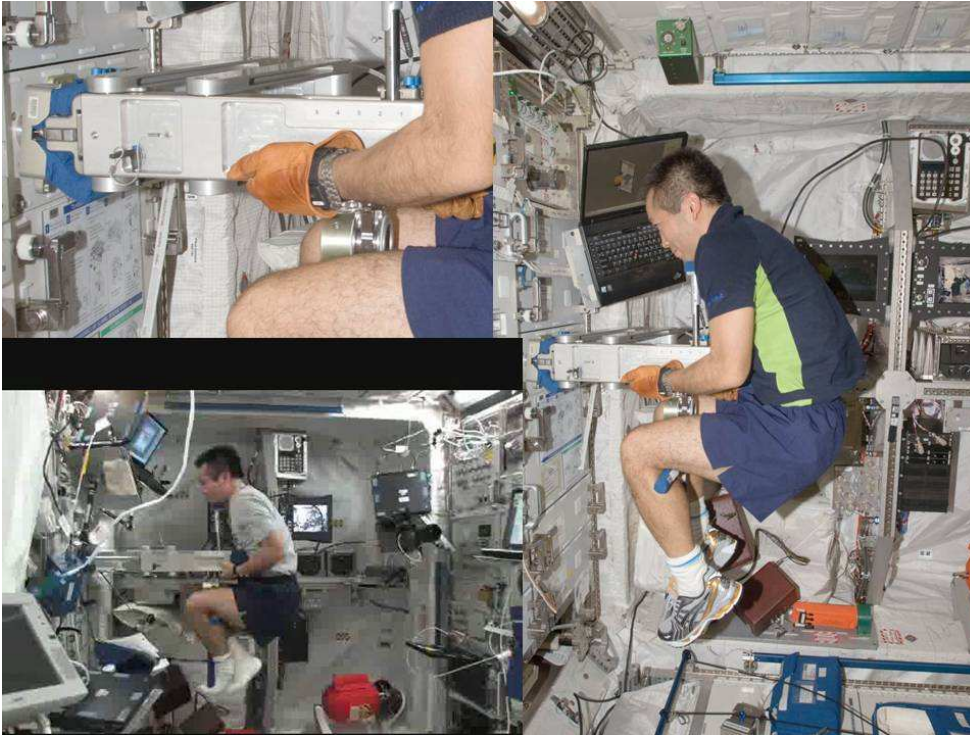
Fig. 13. NASA SLAMMD. Japanese astronaut Koichi Wakata weighs himself with the Human Research Facility's Space Linear Acceleration Mass Measurement Device (SLAMMD) on ISS, 2009.
