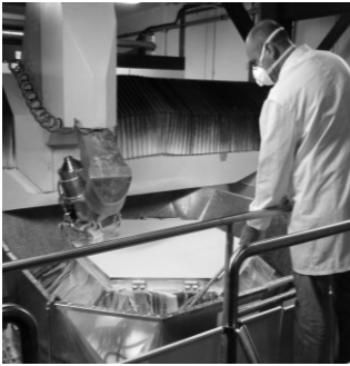
Fig. 1 Segment polishing on the Zeeko IRP1600 machine
