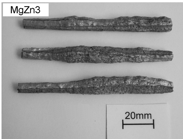
Fig. 11: Foamed specimens for determining the foaming time, alloy MgZn3, heat treated for 2h at 320 °C
