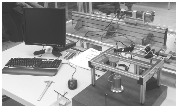
Fig. 47: RFDA MF23 made by the company Integrated Material Control Engineering (IMCE N.V.)
