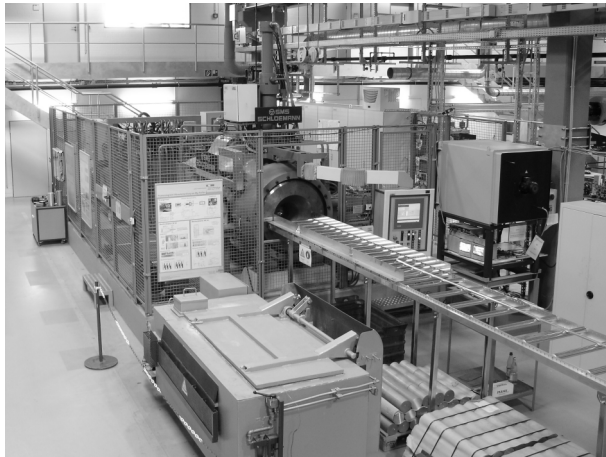
Fig. 51: Institute of Materials Science's (IW) 10 MN extruder (made by the company SMS Meer)
