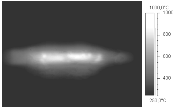
Fig.32: Thermographic image of a surface which is heated by a focused lineal emitter
