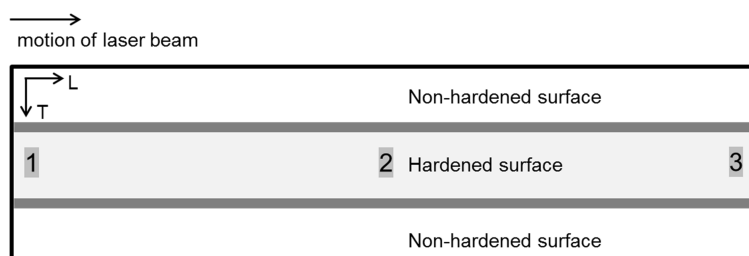
Fig. 1 Drawing of sample surface laser hardened with 20mm wide beam. Numbers 1, 2 and 3 denote irradiated surface area during surface XRD measurements in longitudinal (L) and transverse (T) directions and correspond to beginning (area 1), centre (2) and the end (3) of laser beam path.
