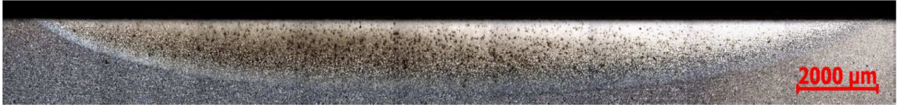
Fig. 2 Microstructure after hardening by 20mm wide laser beam seen on metallographic cross-section.
