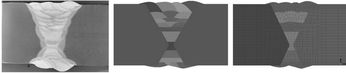
Fig. 4: 30 mm flange connection; macro section (left), derived weld build-up (centre), simplified numerical model (right)
