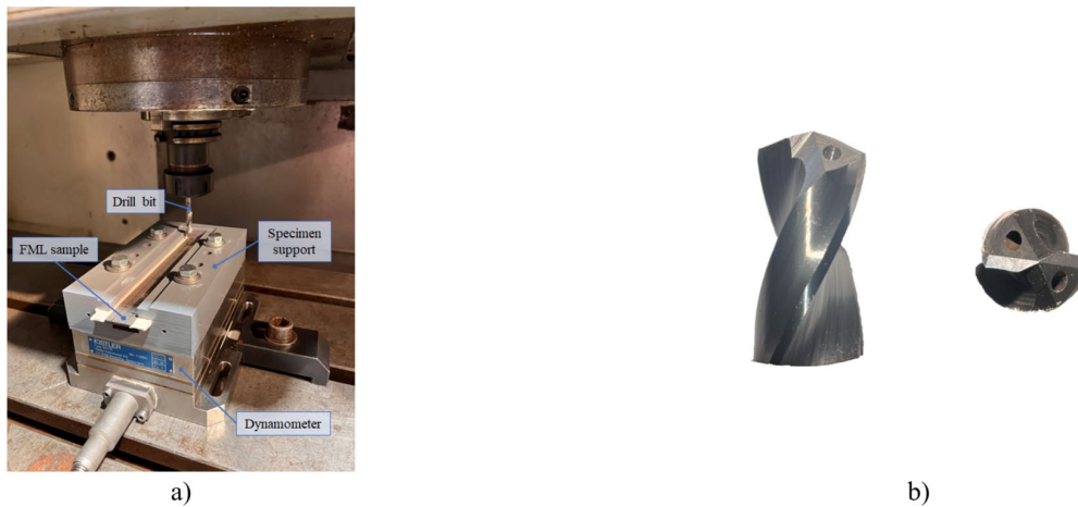
Fig. 2. a) Drilling experimental setup; b) drill bit geometry.
