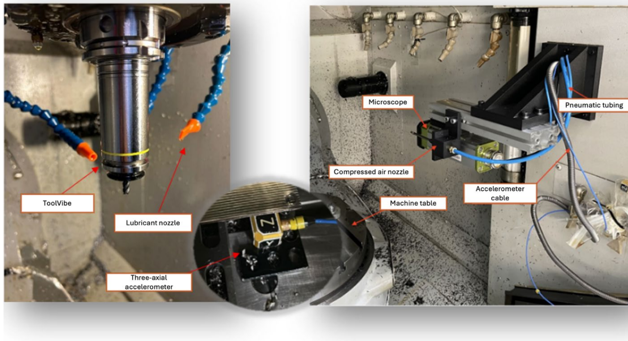
Fig. 1. Sensor configuration adopted during the experimentation.
