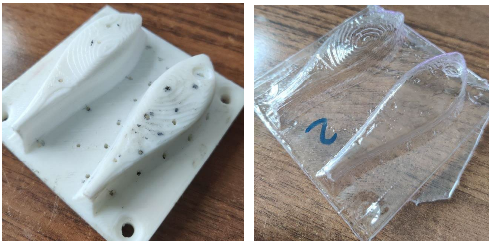
Fig. 2. Surface finishing by sanding and coating (r), result (l) [18].
