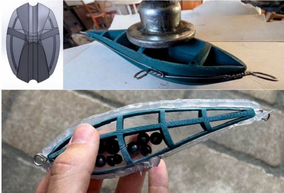
Fig. 3. Joining of lure sample: model of two halves (ur), wire harness (ul), cage, weights, harness, lower shell and sealant (b) [18].
