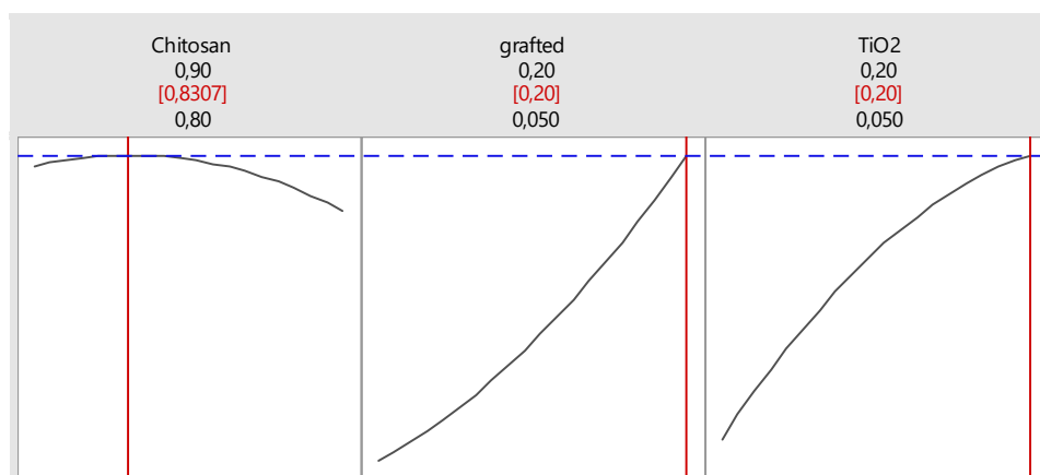
Fig. 2. Solution for the optimum composition of chitosan-grafted cellulose/TiO 2 film on the MB adsorption capacity of the Behnken Design Box.
