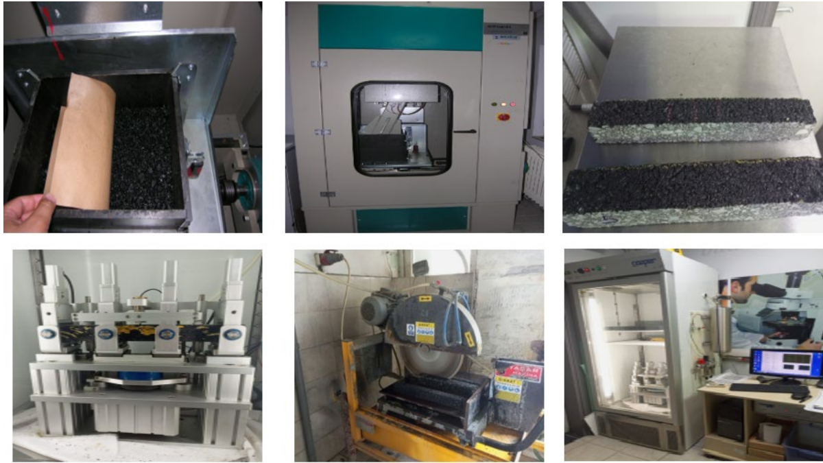
Fig. 4. Some Images of the Four Point Fatigue Test Process
