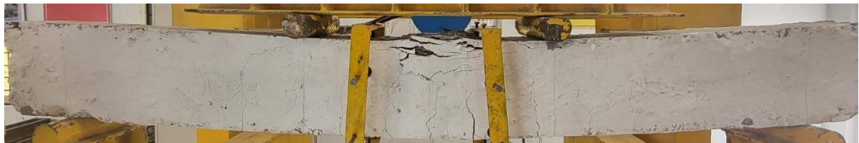
Fig. 5e. Crack Propagation of RC beam using Hybrid Reinforcement and PVA fibers (H30 0.25PVA)
