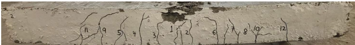
Fig. 5a. Crack Propagation of RC beam using only steel bars(S30 0PVA)
