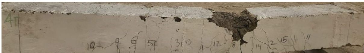
Fig. 5c. Crack Propagation of RC beam using only GFRP bars (F30 0PVA)
