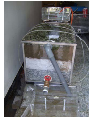
Fig. 6 Vegetated Swales Facility test unit overall.
