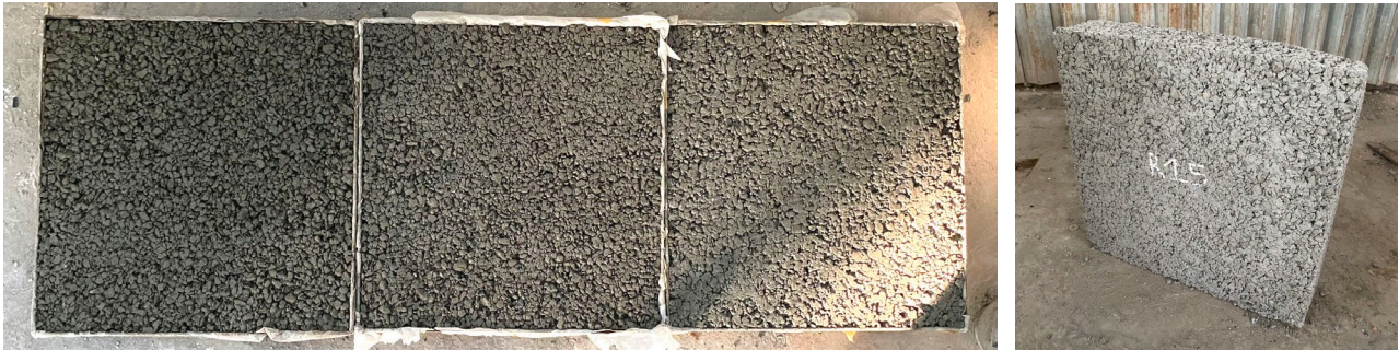
Fig. 1 Casting of pervious concrete samples
