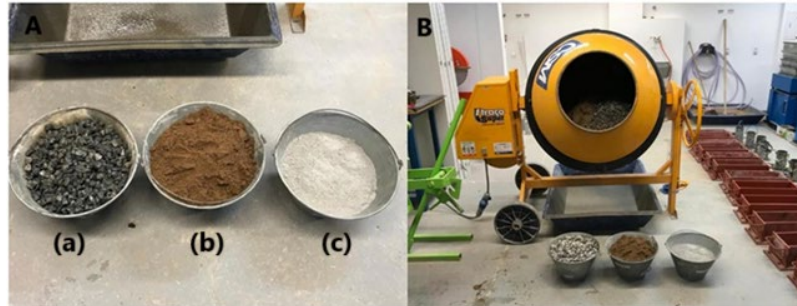
Fig. 1. (A) materials used in preparing the concrete mix (crushed stone (a), sand (b), and cement (c)); (B) mixing materials in an electric concrete mixer.
