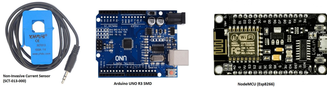
Fig. 2 Key hardware components of IoT-based smart energy monitoring system.
