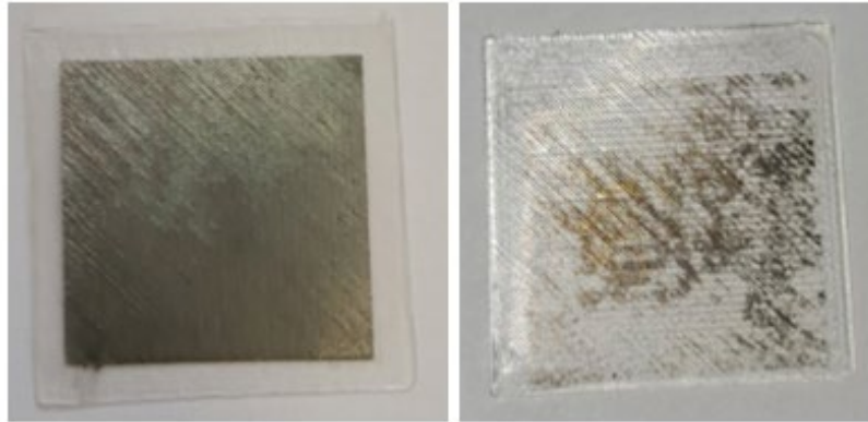
Fig. 15. Inkjet printed sample, before and after the removal of the silicon oil.
