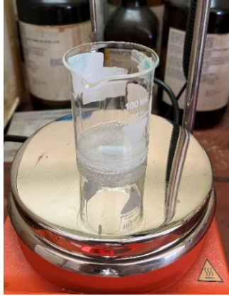
Fig. 4. Stirring of PVDF in DMF and acetone solution.
