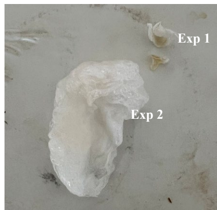
Fig. 5. Foam-like structure of PVDF during both experiments.
