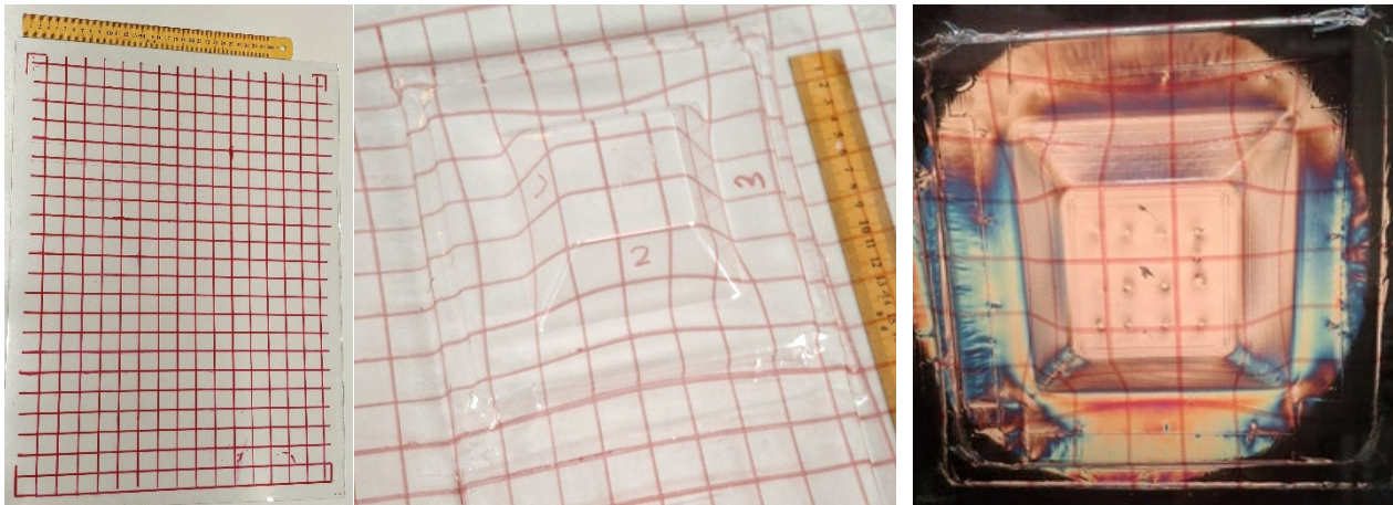
Fig. 20. Undeformed sheet 540 mm × 400 mm with mesh (left), State of deformation of the thermoformed sheet (middle) and orientations in polarized light (right).
