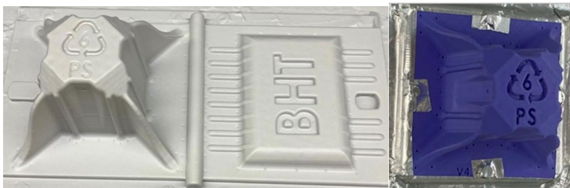
Fig. 1. Example of a thermoformed component produced during a student project (left), massive PLA-mould with 10 mm wall thickness (right), [9].
