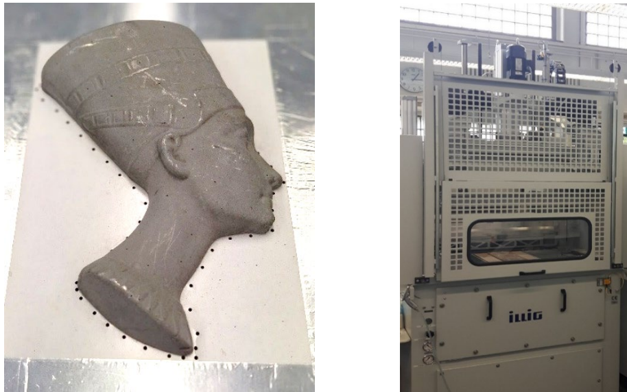
Fig. 3. Conventional aluminum vacuum thermoforming mould (left), Vacuum thermoforming machine Illig UA 100 ed (right).
