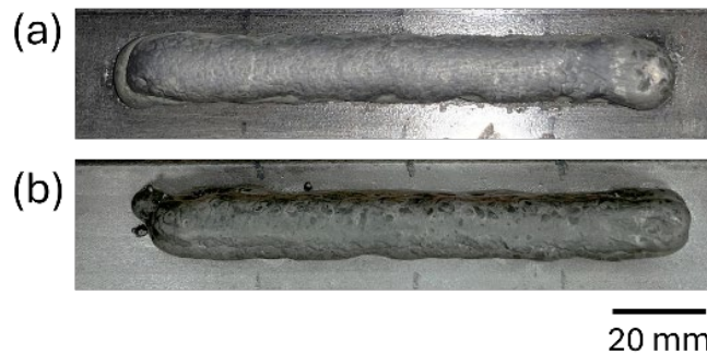
Fig. 3. Top view of the multi-layer walls produced with the two deposition strategies: (a) weave trajectory and (b) linear double-pass.
