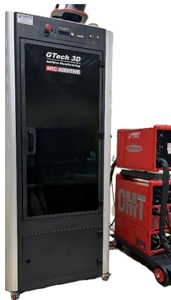
Fig. 1. WAAM setup used for deposition.
