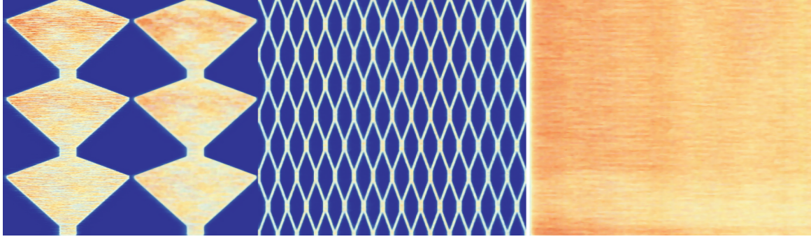
Fig. 6: High-resolution 2D slice renderings obtained from VCS-derived profiles, illustrating planar slicing of a benchmark tree (left), cylindrical unwrapping of a lattice structure (center), and skeleton-based slicing of a curved wall (right).
