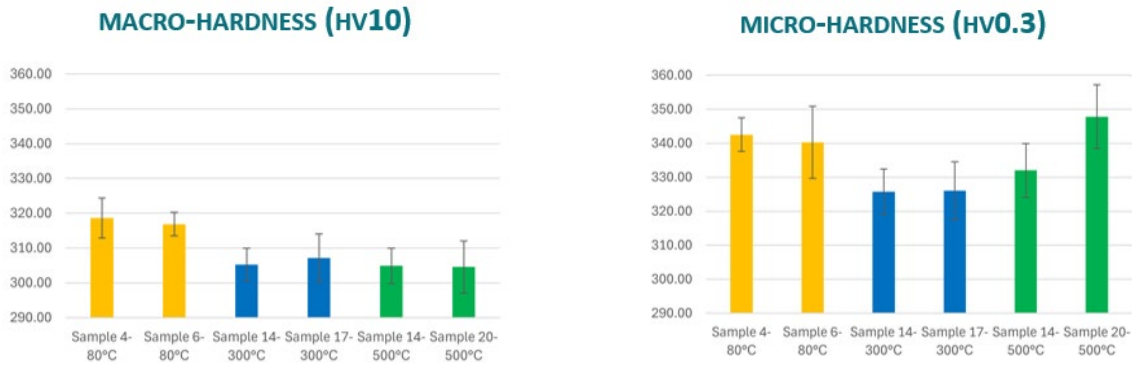
Fig. 5. Overview of hardness as obtained on the full-dense cubes after printing at various preheating temperatures that shows a decreasing trend for the macro hardness with increasing preheating temperature, and a U-shape trend for micro hardness; a) Macro hardness at 10 kg; b) micro hardness at 0.3 kg.
