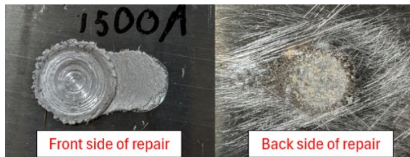
Fig. 5. Representative of the Front (Deposition) and Back (Opposite) Side of a Repair Prior to Milling Flat (Example Shown is from a 1500 A Experiment).
