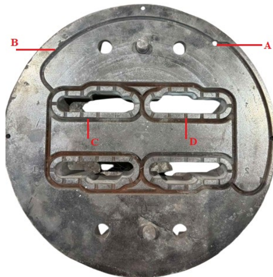
Fig. 1. Liquid nitrogen channels at the aluminum extrusion die
