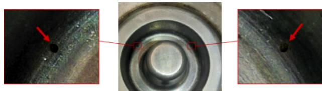
Fig.10. Air vent channels
