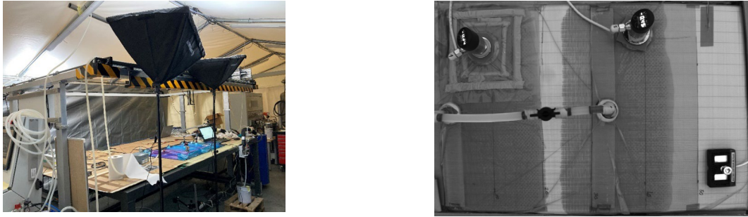
Fig. 4. Infusion test of a plate with camera and lighting - experimental setup (left) and result of the infusion in progress (right)
