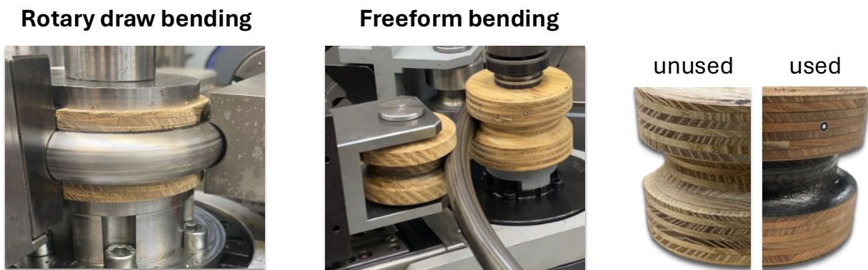
Fig. 2. Wood-based tooling approaches for profile bending. Two common profile bending processes are schematically shown along to a set of wood-based forming tools.
