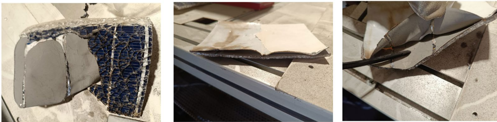
Fig. 4. Post-treatment PV laminate samples.
