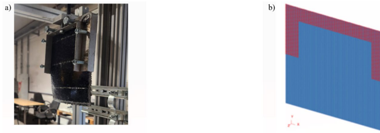
Fig. 3. a) Clamp used for the experimental tests; b) modelled boundary condition.
