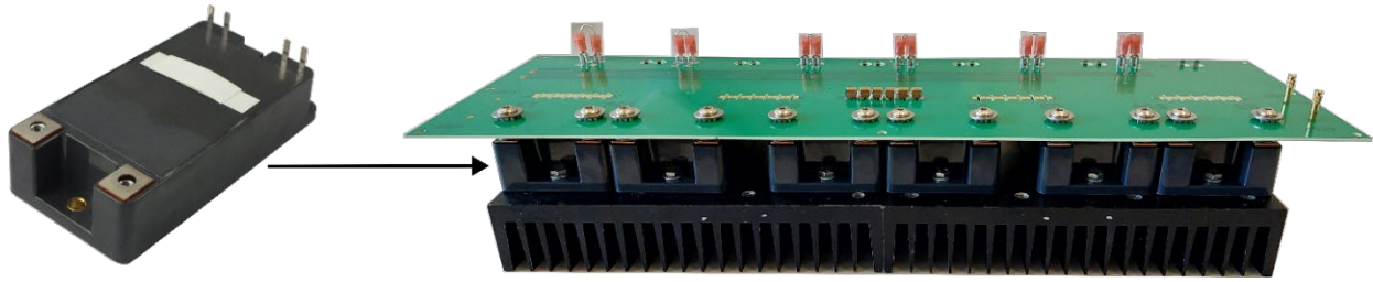
Fig. 1. Left: Single chip 3.3 kV SiC MOSFET in an engineering package filled with silicone gel; right: test stack built up with three half-bridges mounted on air coolers, busbar connection realised with a humidity robust multilayer PCB and additional snubber capacitors for the overvoltage suppression.
