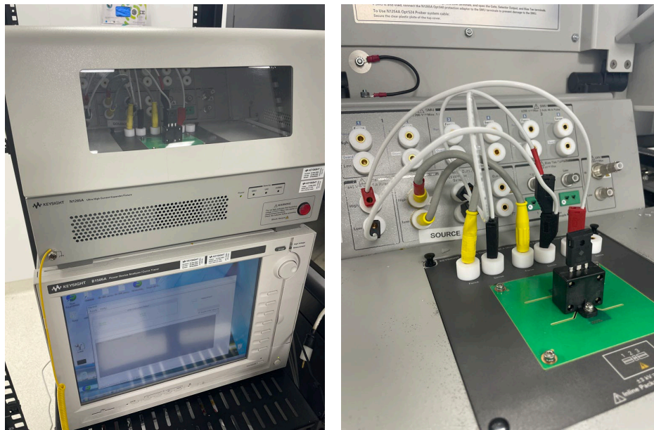
Fig. 1. The Keysight B1505A Power Device Analyzer/Curve Tracer, enabling high-voltage, high-current measurements. For the TO-247 packaged devices, the N1265A expander fixture is used.
