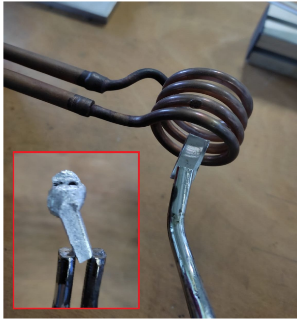
Fig. 4. Foaming test of plain foam with the precursor along the axis of the coil and foamed precursor.
