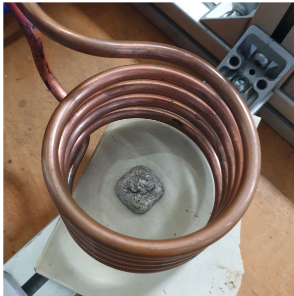
Fig. 5. Foaming test of plain foam with the precursor at the base of the coil.
