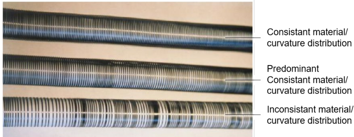
Figure 2: Depiction of the effect of multiple changes of the axial displacement over the length of the coil [8]
