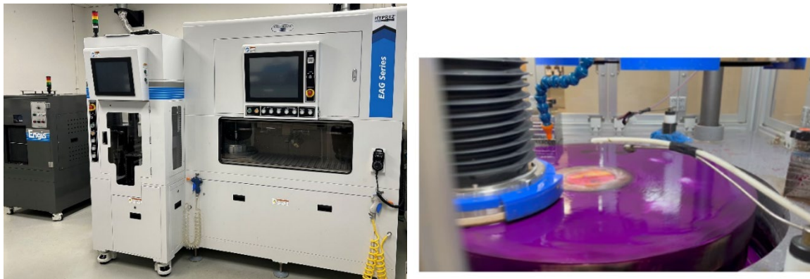
Fig. 1. HYPREZ EAG-28DANX dual spindle, cassette-to-cassette wafering system for 150 to 200mm SiC and EJW-610 CMP machine with HYPREZ SiC pad and slurry.
