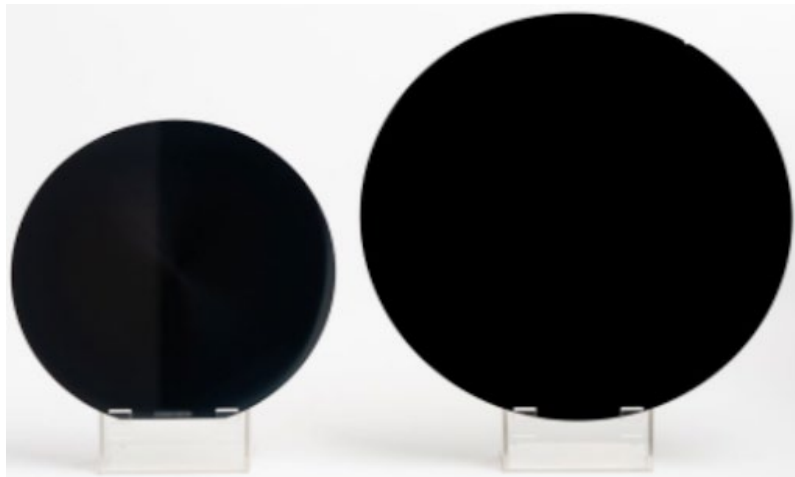
Fig. 2. 150mm & 200mm SmartSiC™ substrate ready for SiC drift epitaxy
