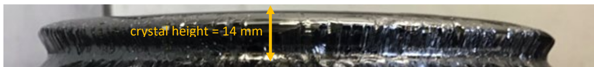
Fig. 3. Example of the side-view of an as-grown 150 mm 4H-SiC (grown using basic hotzone configuration I, cooling channel B and crucible variant #2).
