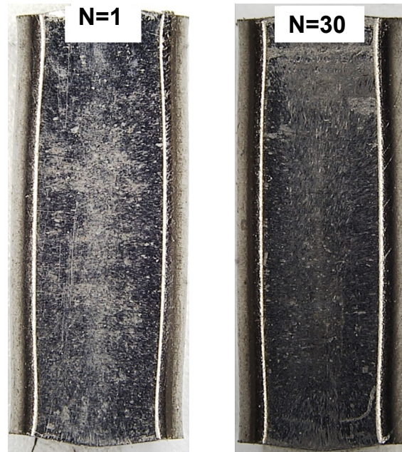
Fig. 4. Comparison of MCSed ACD56 die surfaces at N = 1 and N = 30 .
