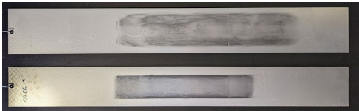
Fig. 8. Sliding tracks on flat strip-draw friction test samples are visible as a grayish mark.
