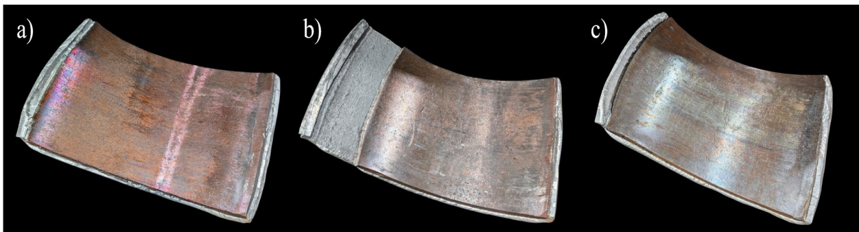
Fig. 14. Experimental results of continuous compound casting and warm rolling with the setup a) – c).
