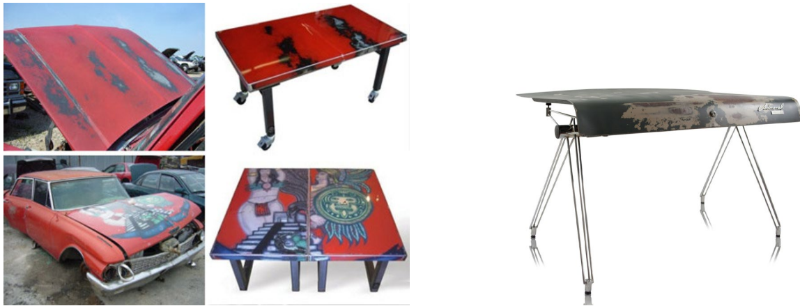
Fig. 2. Examples of products obtained from upcycled automotive sheet metal. From left to right, Tables obtained from scrapped automotive sheets, made by Weld House (Photo by Dornob). A table obtained from an Opel Admiral car, made by Unibro Design.
