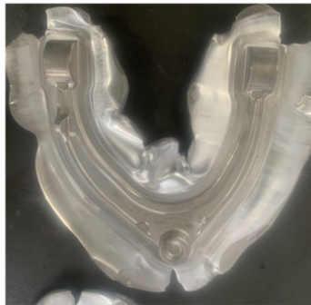
Fig. 9. Forged upper control arm.
