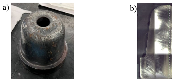
Fig. 1. a) H13 hot forging die employed for the study, and b) slice cut from the die with wire EDM for experimental characterisation.
