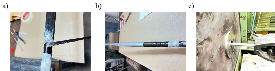
Fig. 2. a) Carbon fiber reinforcement placed along the length and circumference of the inner tube. b) Stacking the two tubes with carbon fiber reinforcement to form a composite. c) The composite drawing process.
