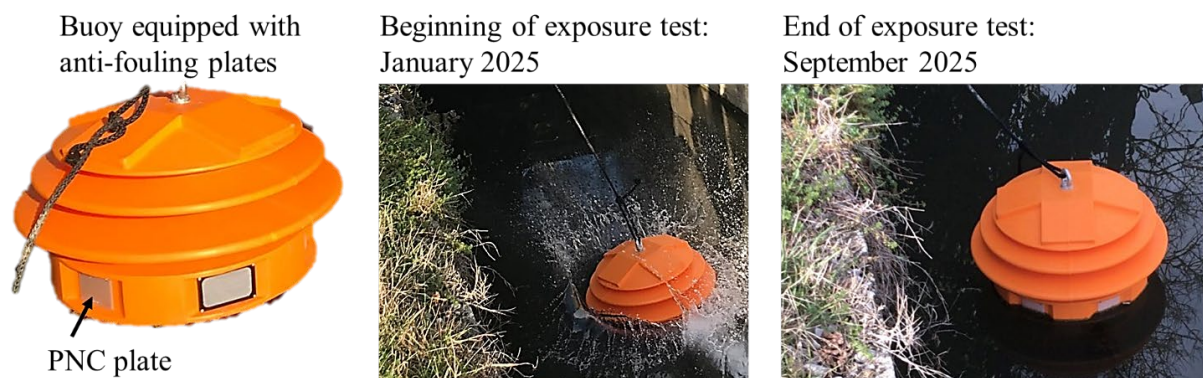
Fig. 3. Positioning of the PNC samples on the smart buoy, by replacing some pyrolytic carbon filters, and exposure in open environment for the experimentation.
