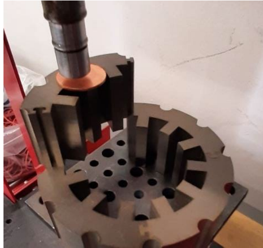
Fig. 2. Joining process of a quarter-segmented stator with T-Form connection geometry
