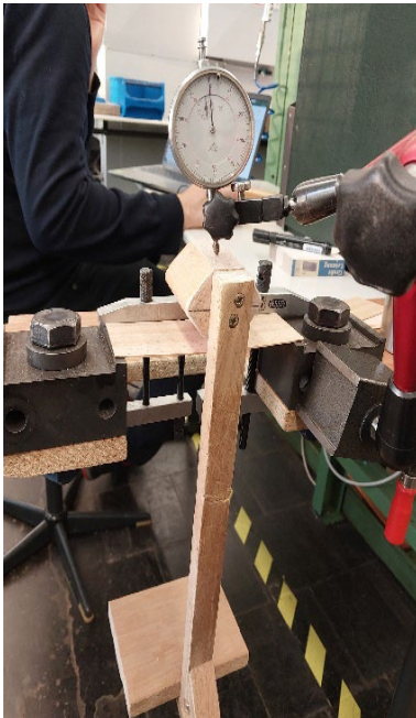
Fig. 14. Test setup for measuring deformation and distance between support, (distance 135 mm).
