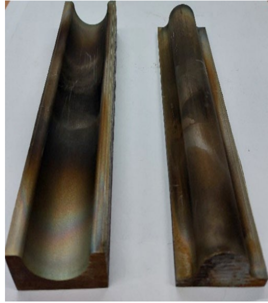
Fig. 9. Used bending mould (WEDM).
