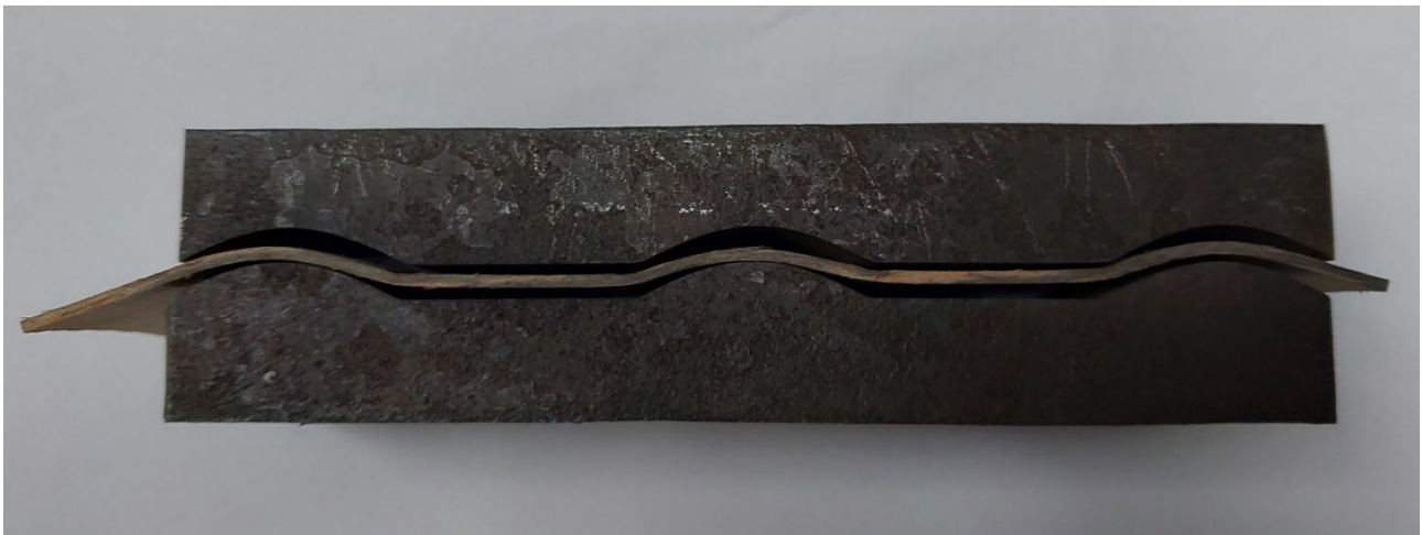
Fig. 20. Spring-loaded component after premature removal from the mould.
