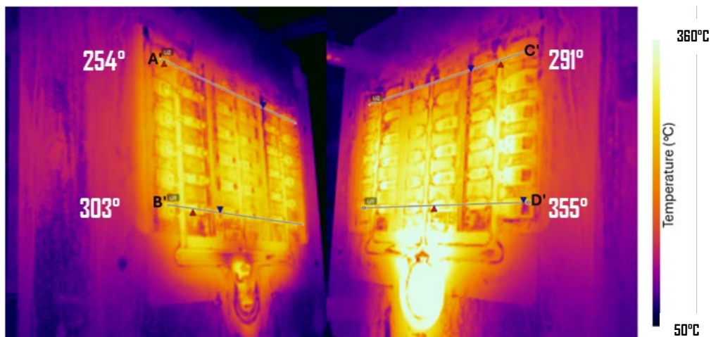
Fig. 9 Infrared thermography of the movable (left) and fixed (right) dies, showing surface temperature distribution at steady-state condition (time instant before the spraying step). Lines A'–D' indicate the paths along which the temperatures were monitored.
