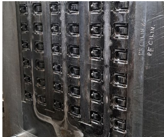
Fig. 3 Metallized regions on the die surface
