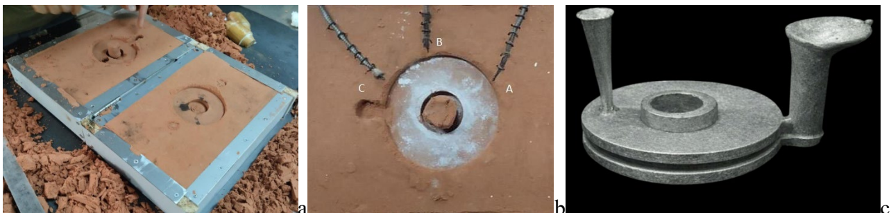
Fig. 5 (a) Mold preparation (b) Thermocouple positions (c) Casting.
