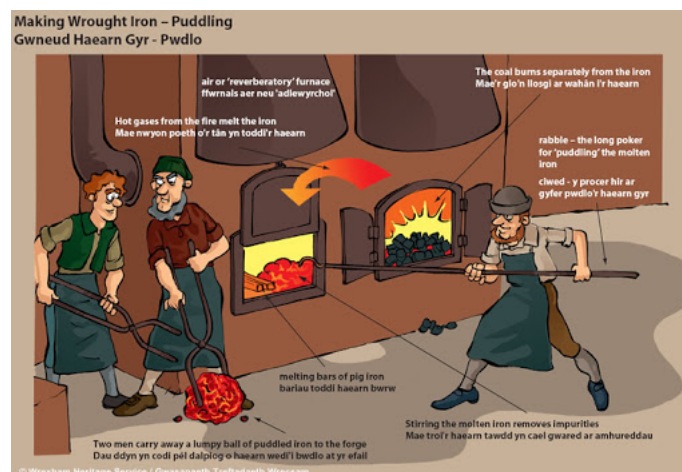
Figure 7. Schematic Illustration of Puddling
