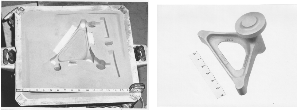
Figure 3. Left) Drag half of a sand mold for a “premium quality” aluminum sand casting, showing chills embedded in the mold. Right) finished casting.
