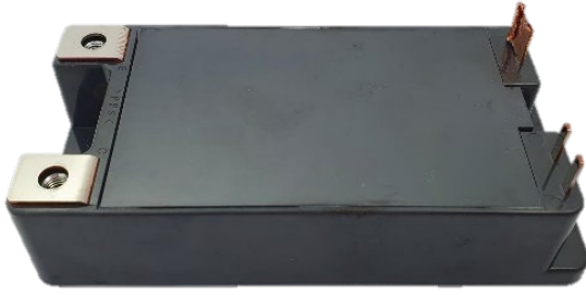
Fig. 1. Image of a device under test. The DUTs feature an AlN substrate, a copper baseplate and were produced by Mitsubishi Electric Corp. as engineering samples. They are fabricated with traction rated materials and produced on the same line as the standard modules. The footprint of the package is 125 mm by 60 mm. The module is populated with 3.3 kV SiC MOSFET chips with a nominal R_{DSon} of 40 m \Omega .
