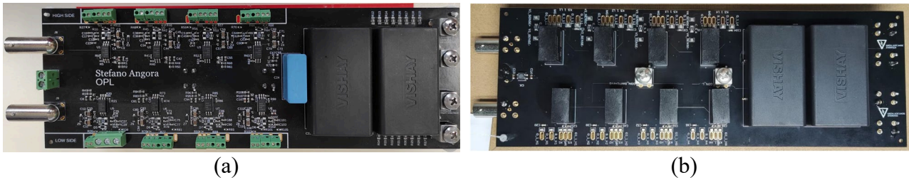
Fig. 2. (a) Top and (b) bottom view of the assembled printed circuit board of the DC-DC converter.
