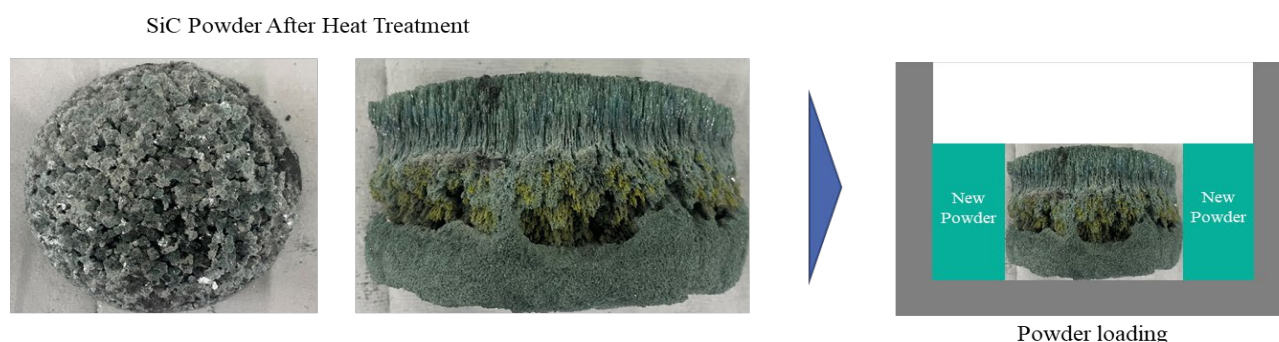
Fig. 2. Photograph of heat-treated recycled powder bulk after the heat treatment and schematic diagram of crucible showing loaded recycled powder bulk.
